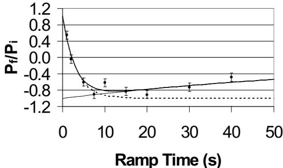
Figure 5: Shows the measured ratio of the final to initial polarization and a fit to the Froissart Stora Formula.
