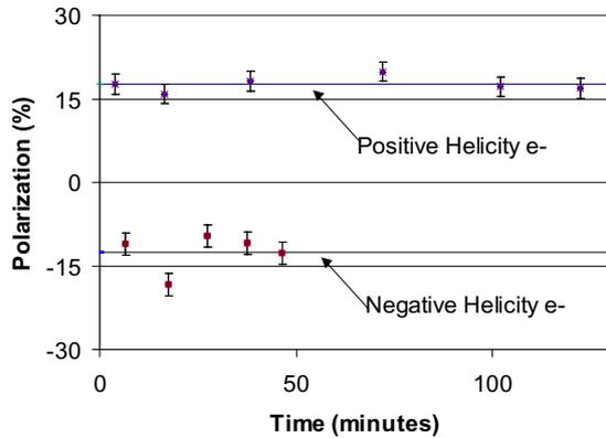
Figure 3: The measured polarization as a function of time the 669 MeV beam was stored in the SHR. The two data sets are for positive and negative helicity electrons.
