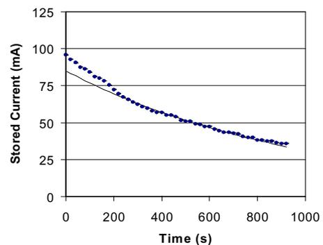
Figure 2: Stored electron current as a function of time. The Siberian Snake was on and the beam energy was 669 MeV for this measurement.
