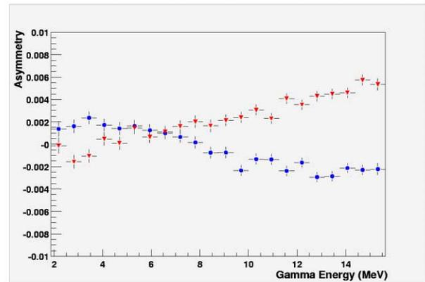
Figure 4: The measured Compton asymmetry for two opposing electron helicity states injected into the SHR. Note the slightly positive offset in the crossing point at 6 MeV indicating a  $10^{-3}$  false asymmetry.
