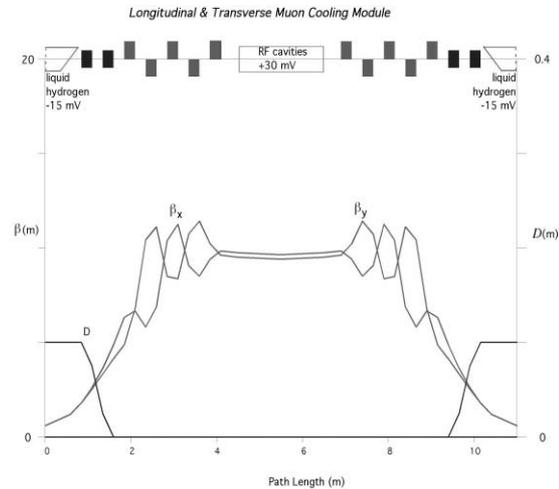
Figure 5. Cooling module of a storage ring cooler.
