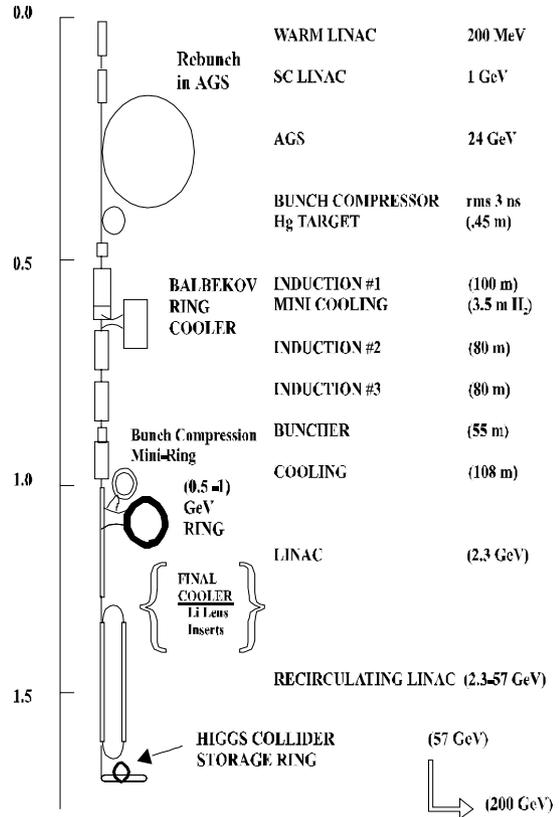
Figure 2. Schema for converting a Neutrino Factory to a Higgs Factory.
