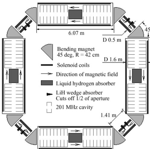
Figure 4. The Balbekov cooling ring.
