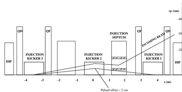
Figure 3: Injection straight section in VLER with a pulsed orbit bump.
