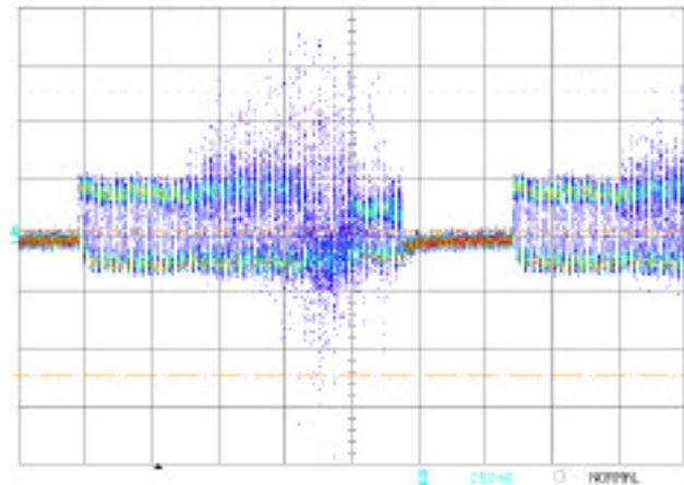
Figure 3: E+ correction signal with 45/60 bunches (~400mA)
