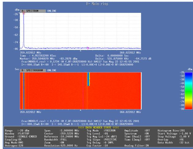
Figure 5: E- beam: no vertical oscillation (feedback on)
