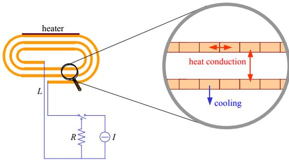
Figure 1: Quench Calculation model.
