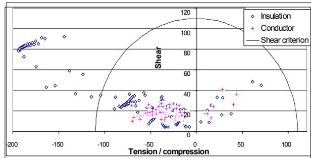
Fig. 7: Von Mises criterion of thermal stress and strain for a 1m long magnet after 100ms.
