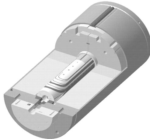
Figure 1: Two-layer shell-type Nb<sub>3</sub>Sn dipole model
