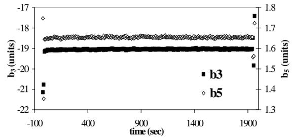
Figure 7:  $b_3$ ,  $b_5$  near the injection plateau. The current ramp stops at  $t=0$ . The first 3 measurements after ramping begins again are also plotted.
