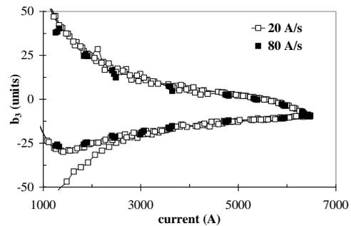
Figure 3: Measured  $b_3$  at different ramp rates
