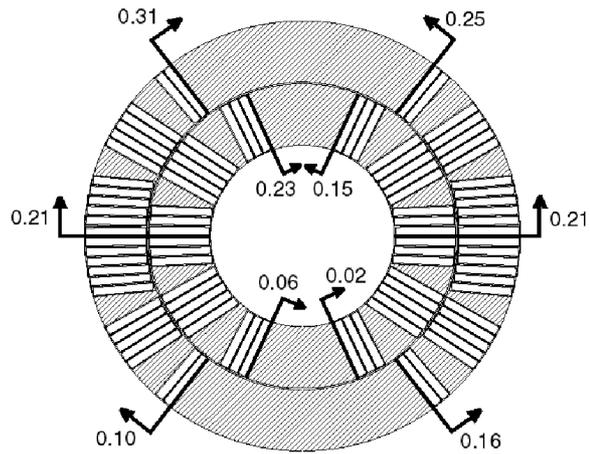
Figure 2: Model of HFDA02 as built which reproduces the measured low order field harmonics. Shifts shown are in units of mm.
