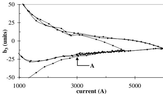
Figure 6:  $b_3$  measured during an accelerator cycle
