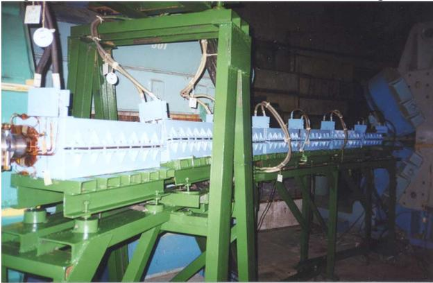
Fig. 5: The fragment of beam transfer line UK/U10 with bending magnets path.
