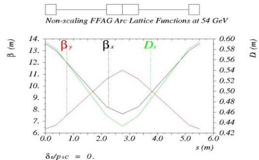
Figure 2. Lattice functions at 54 GeV for a 16-64 GeV non-scaling FFAG.
