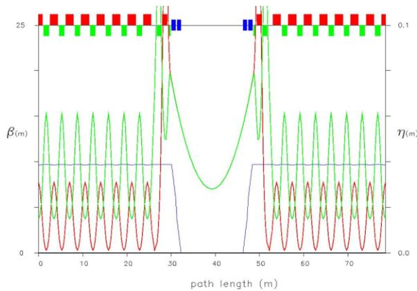
Figure 1. A sector of the 16-64 GeV scaling FFAG showing the 14 m dispersion-suppressed drift.
