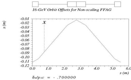
Figure 3. 16-GeV (top) and 64-GeV (bottom) orbit amplitudes for a 16-64 GeV non-scaling FFAG.
