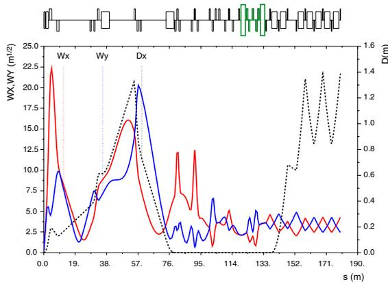
Figure 2: Lattice functions of the electron ring interaction region.
