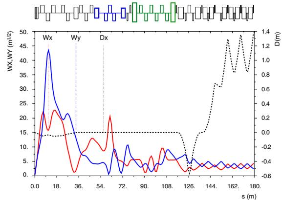
Figure 3: Lattice functions of the proton ring interaction region.
