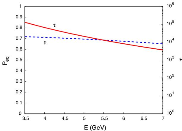
Figure 4: The equilibrium degree of polarization and the spin relaxation time as functions of the electron energy.
