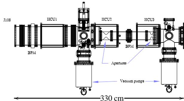
Figure 1: Elevation view of the beam cleanup zone. HCU1-3 are solenoids, J108 is the last solenoid in the injector block.
