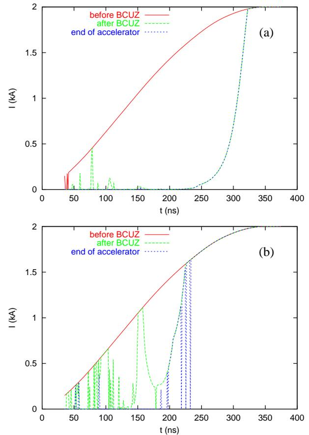
Figure 3: Current waveforms before the BCUZ, after the BCUZ and at the end of the accelerator for (a) cleanup tune and (b) smooth tune.
