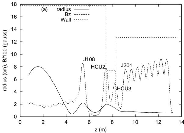
Figure 2: Beam-body tune vs.  $z$  for the “head-cleanup” tune. Edge radius, axial magnetic field, and wall radius are shown.
