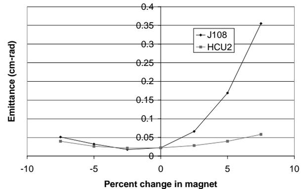
Figure 6: Emittance at the end of DARHT-2 as a function of the change in magnets J108 and HCU2 for the cleanup tune.
