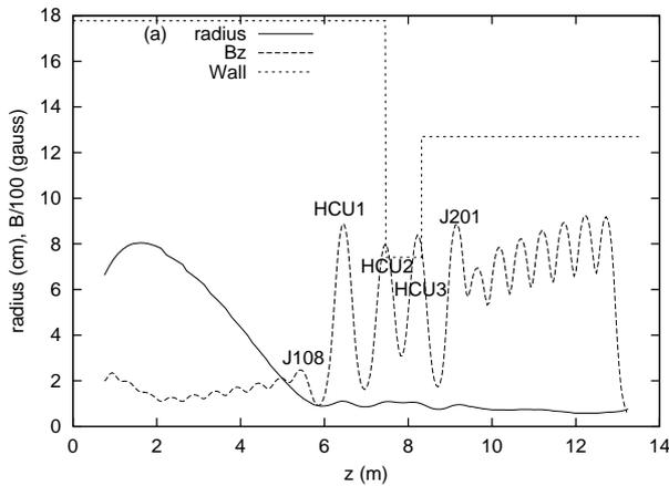
Figure 4: Beam-body tune vs.  $z$  for the “smooth” tune. Edge radius, axial magnetic field, and wall radius are shown.
