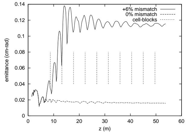
Figure 5: Comparison of emittance for matched and mismatched (+6% change in J108) transport.
