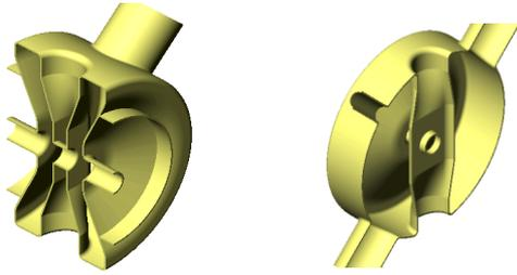
Figure 3: Cutaway of 2-Gap Spoke Resonator.
