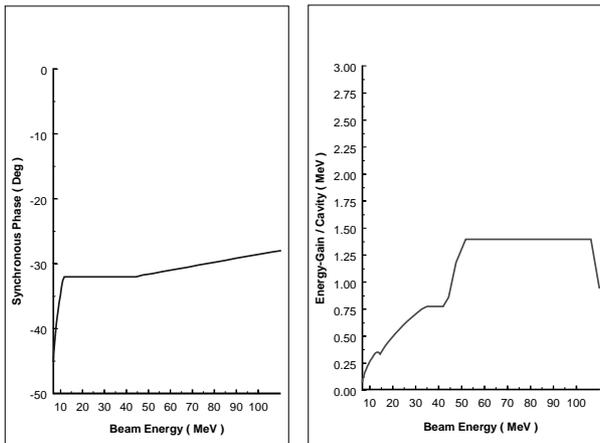
Figure 5: Synchronous phase and energy-gain ramps.
