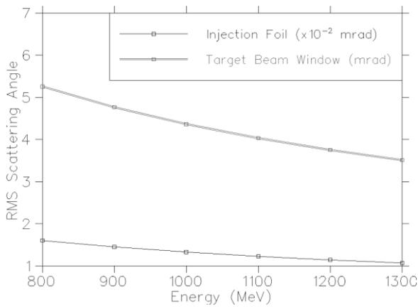
**Figure 4:** RMS multiple scattering angles as a function of energy for proton beam window in RTBT which is 4 mm thick made of inconel and injection carbon foil  $300\mu\text{g}/\text{cm}^2$ .
