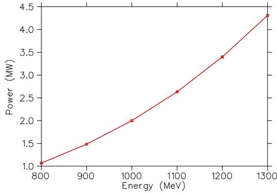
**Figure 2:** Beam power as function of injection energy in the accumulator ring for space charge tune shift of 0.15.
