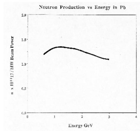
**Figure 5:** Neutron yield per MW of beam power for a lead target.
