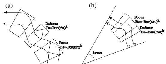
Figure 2: Lattice of Radial Sector Type FFAG (a) Original Radial Sector (b) Triplet Radial Sector
