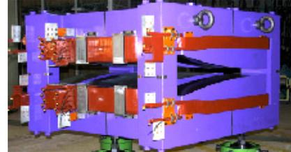
Figure 9: "Return-Yoke Free" Magnet for 150MeV FFAG synchrotron
