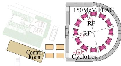
Figure 1: Layout of 150MeV FFAG synchrotron
