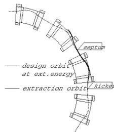
Figure 10: Beam Extraction Scheme
