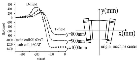
Figure 4: Typical Field Measurement Results of R&D Magnet
