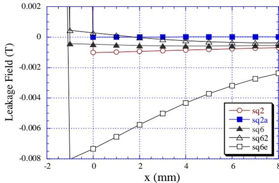
Figure 2: Leakage fields of direct-drive septum magnets. The outer surfaces of the septa were located at  $x = 0$  for sq2 and sq2a, and  $x = -1.0$  for sq6, sq62, and sq6e. The current  $I_s$  was varied: sq2 ( $I_s$  not changed); sq2a (0.16% of  $I_s$  diverted to CS); sq6 (0.27% of  $I_s$  to  $S_2$ , thicker part of S near the magnet pole); sq62 (0.76% of  $I_s$  to  $S_2$ ); and sq6e (0.3-mm air gap between the septum and magnet core).
