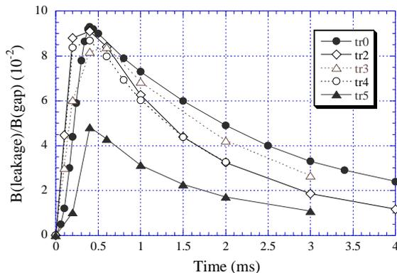
Figure 5: Leakage fields as a function of the time from the start of the current pulse were calculated for eddy-current septum magnets with  $\omega_0\tau_1 = 2$  and 2-mm septa. tr0: Cu septum, from Halbach's model for  $a_1=10$ . tr2: Cu septum for  $a_1=10$ . tr3: Cu-Fe septum for  $\mu_r = 20$  and  $a_1=20$ . tr4: Cu septum without beam chamber. tr5: nonlinear calculation for Cu-Fe septum without beam chamber.
