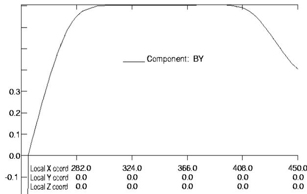
Fig.4: Vertical induction field along horizontal direction
