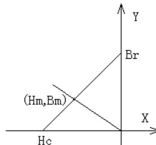
Figure 2. The  $B_r - H_c$  curve of PM Material
