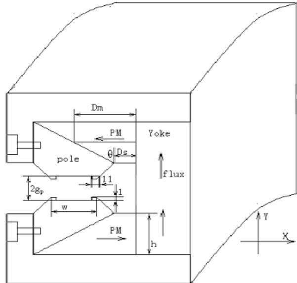
Figure 1. The Novel PM Dipole Configuration
