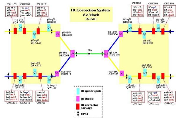
Figure 1: Schematics of one of the RHIC IR's
