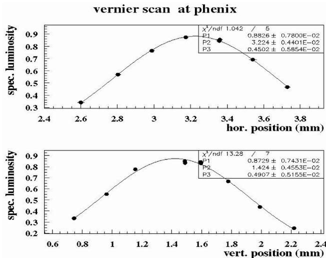
Figure 2: Vernier luminosity scan at the Phenix Ir.
