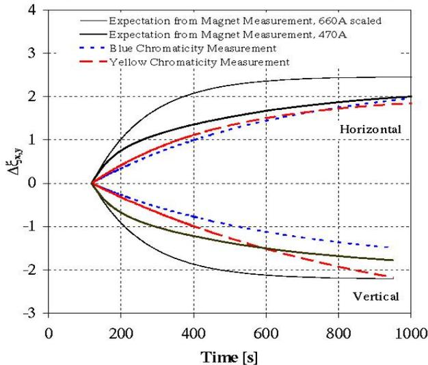
Figure 5: Comparison of measured chromaticity evolution and prediction from persistent currents magnet data.
