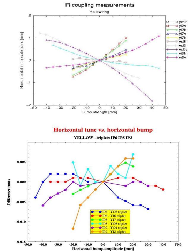
Figure 3: Orbit rms and Tunes shifts as a function of horizontal bump amplitude at several RHIC IR's.
