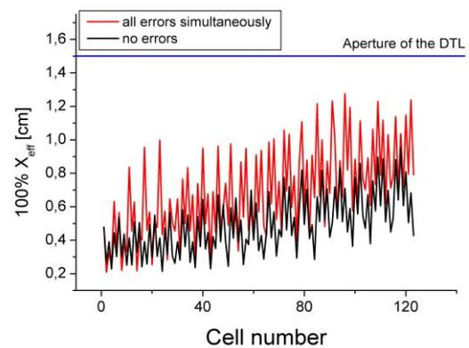
Figure 2: 100% effective beam size in the X-Cell-plane of the DTL with and without combined quadrupole + rf field errors.
