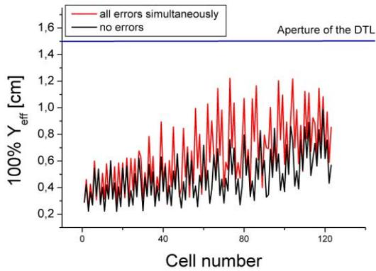
Figure 3: 100% effective beam size in the Y-Ncell-plane of the DTL with and without combined quadrupole + rf field errors.
