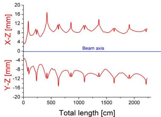
Figure 5: 99% transverse effective beam envelopes of the IH-DTL as a function of the total length.
