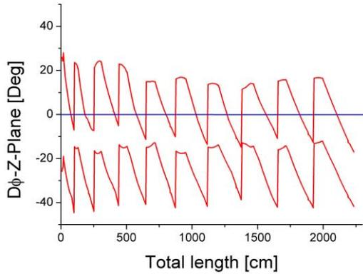
Figure 7: Phase spread of the IH-DTL as a function of the total length.
