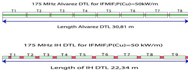
Figure 4: Scaled scheme of the actual Alvarez DTL and IH-type DTL for IFMIF.
