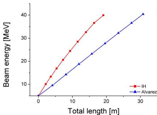
Figure 9: Energy gain of both structures as a function of the total length.
