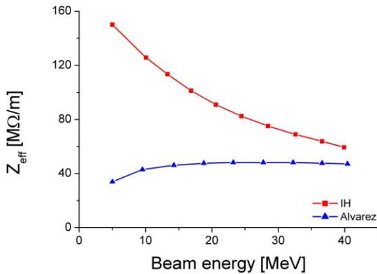
Figure 8: Effective shunt impedances of both structures as a function of the beam energy.
