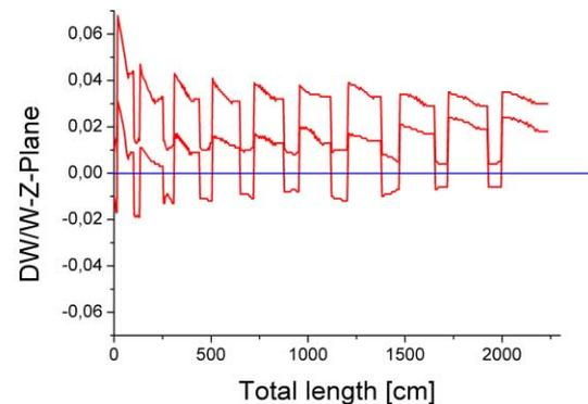
Figure 6: Energy spread of the IH-DTL as a function of the total length.
