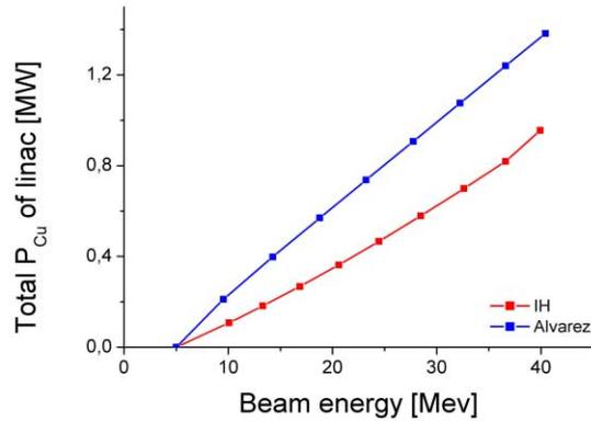
Figure 10: Sum of the rf copper power losses per tank of both structures as a function of the beam energy.
