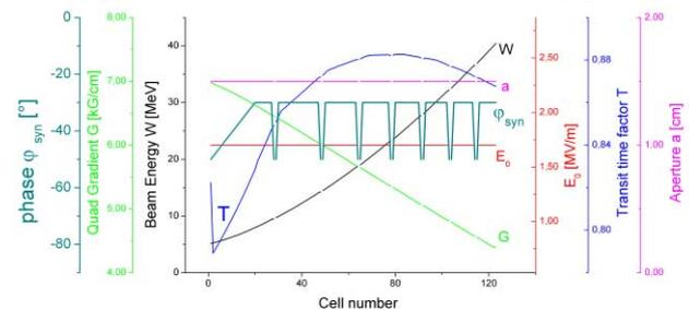
Figure 1: Structure parameter of the DTL as a function of the beam energy.
