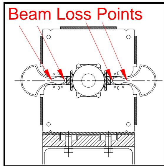
Figure 1: Beam loss points in the VLHC Stage-1 magnet.
