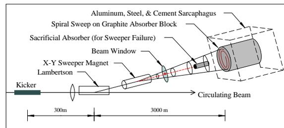
Figure 3: Schematic layout of beam abort channel.
