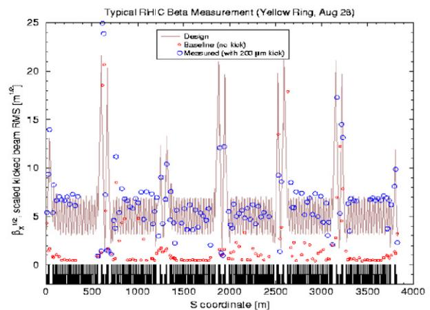
Figure 1: Measured -o- and predicted  $\beta_x$  betatron function in the horizontal plane.
