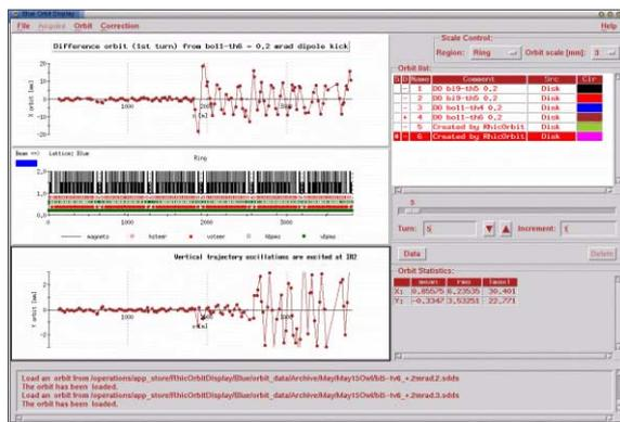
Figure 1: The betatron coupling sources at IRs were observed during the difference orbit RHIC optics measurements.
