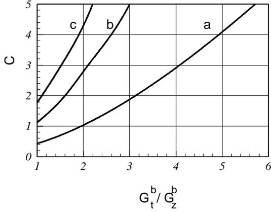
Fig. 1. Coefficient  $C$  in bunch shape for  $\varphi_s = -30^\circ$  as a function of ratio of transverse and longitudinal gradients of space charge field of the beam: a)  $\gamma = 1$ , b)  $\gamma = 3$ , c)  $\gamma = 6$ .
