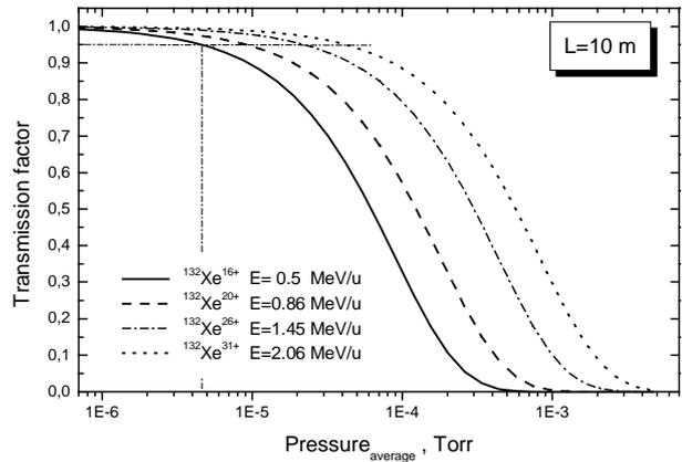
Figure 8: The transmission efficiency of  $^{132}\text{Xe}^{16+}$ ,  $^{132}\text{Xe}^{20+}$ ,  $^{132}\text{Xe}^{26+}$ , and  $^{132}\text{Xe}^{31+}$  ions in the extracted beam channel.
