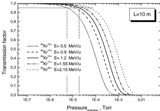
Figure 7: The transmission efficiency of  $^{84}\text{Kr}^{10+}$ ,  $^{84}\text{Kr}^{13+}$ ,  $^{84}\text{Kr}^{15+}$ ,  $^{84}\text{Kr}^{17+}$  and  $^{84}\text{Kr}^{20+}$  ions in the extracted beam channel (of length  $L=10$  m) of the CI-100 cyclotron.
