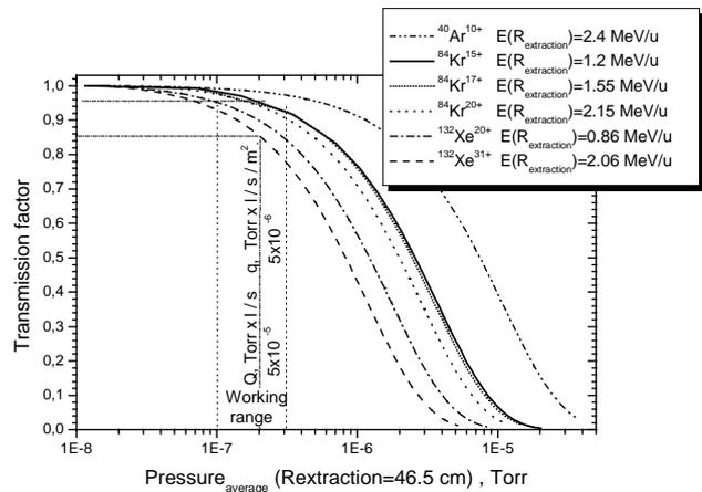
Figure 5: The transmission efficiency of  $^{40}\text{Ar}^{10+}$ ,  $^{84}\text{Kr}^{15+}$ ,  $^{84}\text{Kr}^{17+}$ ,  $^{84}\text{Kr}^{20+}$ ,  $^{132}\text{Xe}^{20+}$  and  $^{132}\text{Xe}^{31+}$  ions in the CI-100 cyclotron up to the extraction radius  $R_{\text{extr}}=46.5$  cm.
