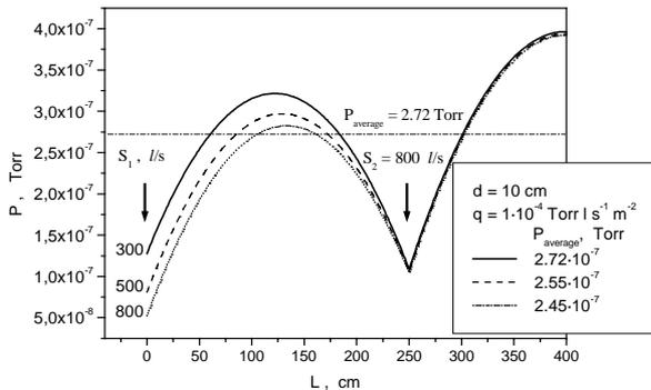
Figure 2: The pressure distribution along the ion guide pipe of the axial injection system for three variants of the pumping speed of the first vacuum pump: 300, 500 and 800 l/s.
