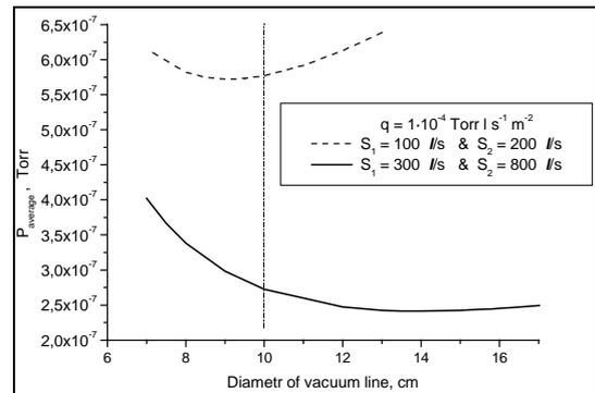
Figure 4: The dependence of the average pressure in the ion guide pipe on the diameter under following pumping conditions: 1)  $S_1=100$  l/s and  $S_2=200$  l/s, 2)  $S_1=300$  l/s and  $S_2=800$  l/s.
