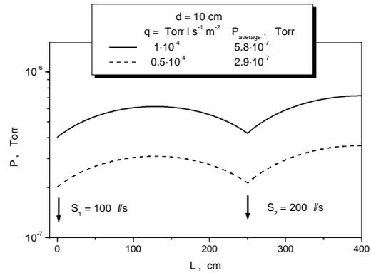
Figure 3: The pressure distribution in the ion guide pipe ( $\varnothing$  10 cm) of the axial injection system for pumping speeds  $S_1=100$  l/s,  $S_2=200$  l/s, under two values of the gas loading:  $q_1=0.5 \cdot 10^{-4}$  Torr $\cdot$ l $\cdot$ s $^{-1}$  $\cdot$ m $^{-2}$  and  $q_2=1 \cdot 10^{-4}$  Torr $\cdot$ l $\cdot$ s $^{-1}$  $\cdot$ m $^{-2}$ .
