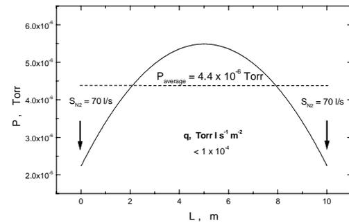
Figure 9: The pressure distribution over the extracted beam channel (of length  $L=10$  m) that is pumped by two pumps with effective speed of  $\text{N}_2$  pumping  $S_1=S_2=70$  l/s.
