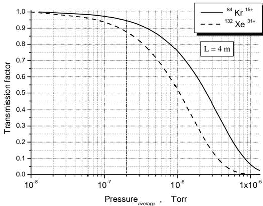
Figure 1: The transmission efficiency in the channel of axial injection system.
