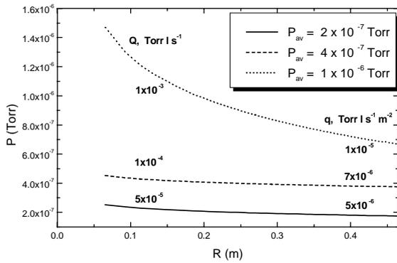
Figure 6: The radial pressure distribution in the cyclotron vacuum chamber under different gas loading conditions for the gas flow in the cyclotron central region  $Q$ , Torr-l/s and specific outgassing rate  $q$ , Torr-l-s<sup>-1</sup>-cm<sup>-2</sup>:
