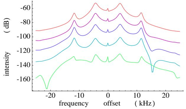
Figure 1: Simulated beam response functions  $T_{955}$ ,  $T_{1855}$ ,  $T_{3655}$ ,  $T_{5555}$ , and  $T_{13555}$  (top to bottom) for a fully stretched 500-mA bunch in the National Synchrotron Light Source (NSLS) Vacuum Ultra-Violet (VUV) ring. Realistically detuned main- and harmonic-cavity impedances are included in the simulation. The vertical scale has an arbitrary scale factor. Machine parameters are given in Table 1.
