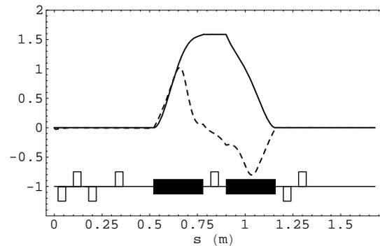
Figure 2: Lattice function  $\mathcal{H}_x$  (solid line) in units of 10 cm and  $\phi_{Bx}$  (dimensionless).
