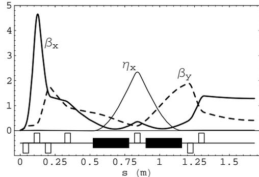
Figure 1: Lattice functions;  $\beta$ -functions are in m,  $\eta_x$  is in units of 10 cm.
