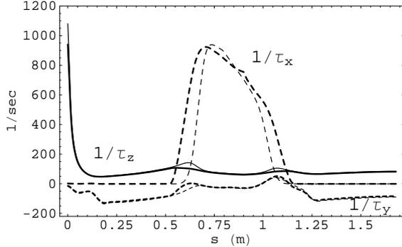
Figure 3: Local IBS growth rates along the lattice. Thick lines refer to calculation done according to Bjorken-Mtingwa; thin lines are calculated according to Piwinski. The vertical growth rate  $1/\tau_y$  is magnified by a factor 100.
