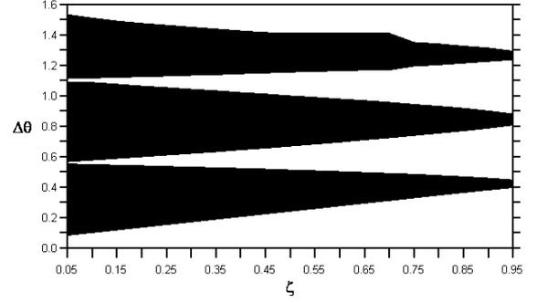
Figure 3: Plot of stable (white) and unstable (black) regions in the parameter space for a periodic wobbling sheet beam.
