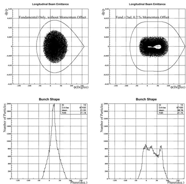
Figure 1: The beam emittance and the bunch shape at the injection in 3 GeV PS.
