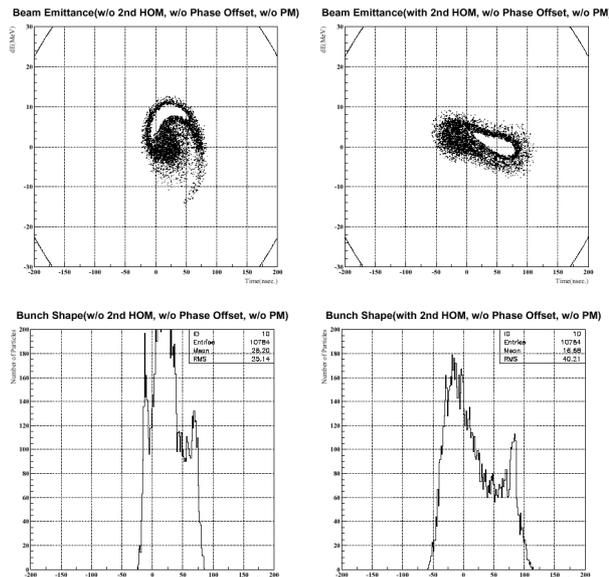
Figure 3: The beam emittance and the bunch shape at the extraction in 3 GeV PS from the view point of 2nd higher harmonics.
