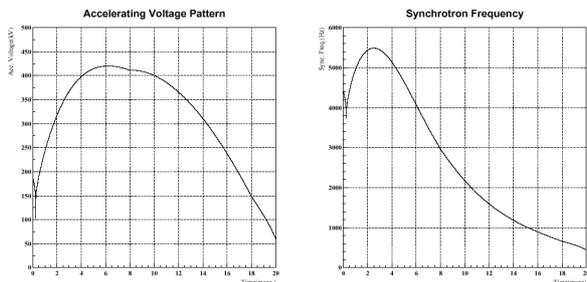
Figure 2: The accelerating voltage pattern and the synchrotron frequency at 3 GeV PS.
