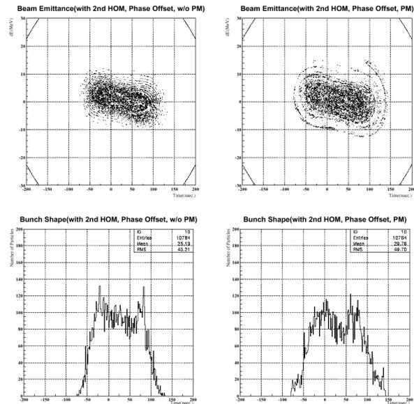
Figure 4: The beam emittance and the bunch shape at the extraction in 3 GeV PS from the view point of phase modulation.
