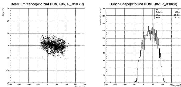
Figure 5: The beam emittance and the bunch shape at the extraction in 3 GeV PS including beam loading compensation.
