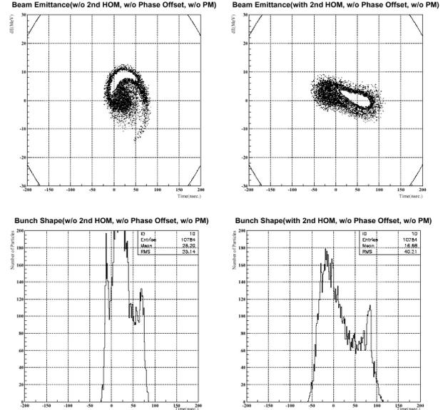
Figure 3: The beam emittance and the bunch shape at the extraction in 3 GeV PS from the view point of 2nd higher harmonics.
