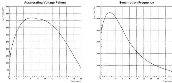
Figure 2: The accelerating voltage pattern and the synchrotron frequency at 3 GeV PS.
