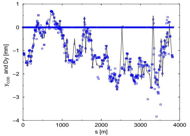
Figure 7:  $y_{COD}$  (solid line) and vertical quad errors ( $\circ$ )
