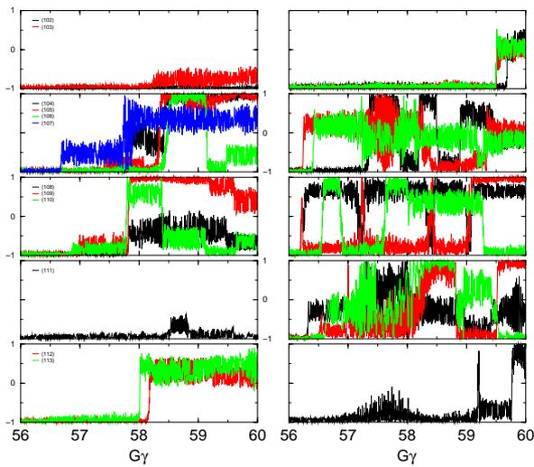
Figure 2: Longitudinal component of the spin at SNAKE2 for runs at various tunes. Orbit 2.3 mm
