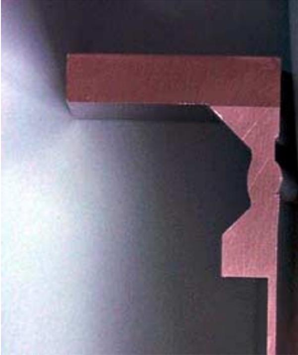
Figure 3: Welding joint between the ID VC and the end box.
