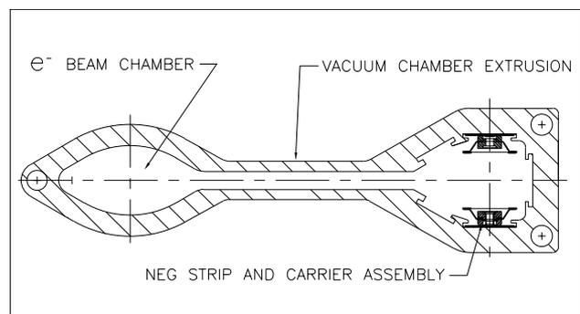
Figure 1: APS vacuum chamber cross section.
