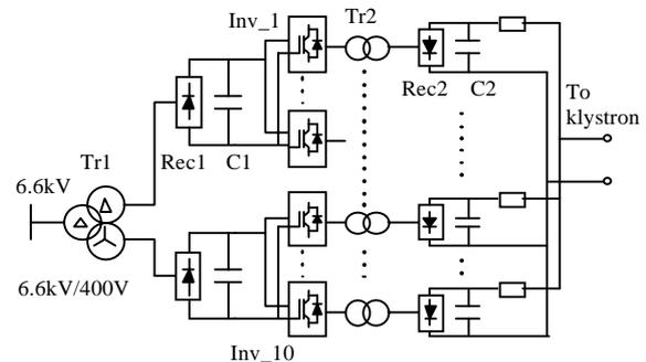
Figure 1: Configuration of a crowbarless power supply.
