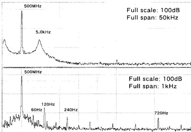
Figure 3: Side bands of the rf frequency of the beam signal, point(3) of Fig.2.
