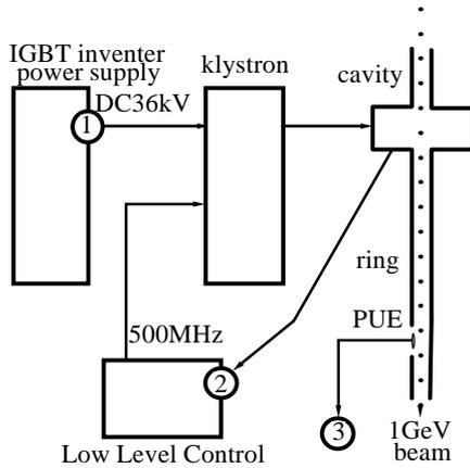
Figure 2: The ripple of DC voltage was measured at the point (1). The phase error of the 500MHz in the cavity was measured at the point (2), PLL signal of the low level control. The phase ripple of the beam is measured using the beam signal picked up from an electrode set at the beam pipe, that was the point (3).
