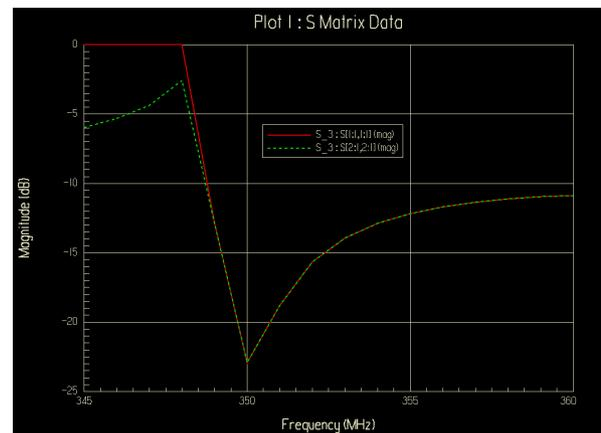
Figure 6. Return loss versus the frequency.
