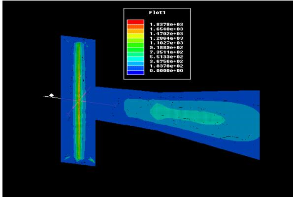
Figure 7. Electric field distribution in the RFQ and input RF coupler
