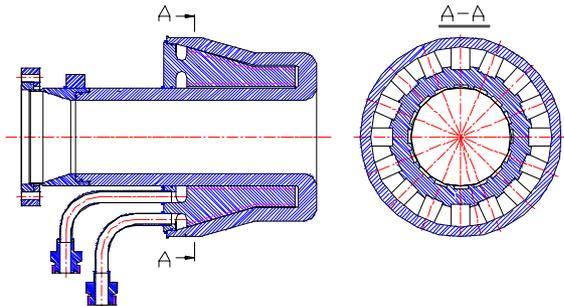
Figure 4: Cuneate cooling structure of the nose
