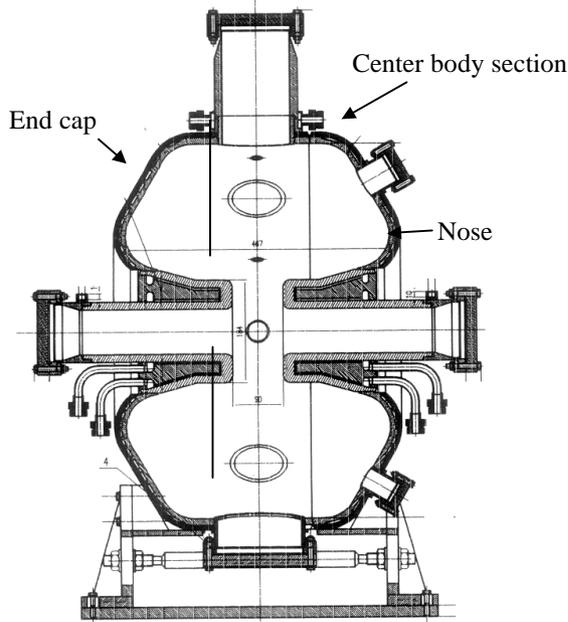
Figure 1: The designed cavity of HLS
