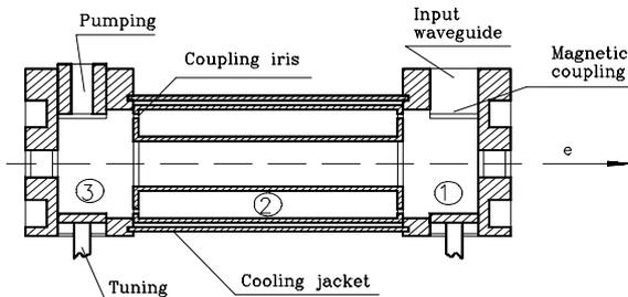
Figure 1: The S-band buncher.
