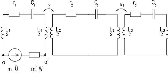
Figure 2: Electric circuit representation of the buncher.
