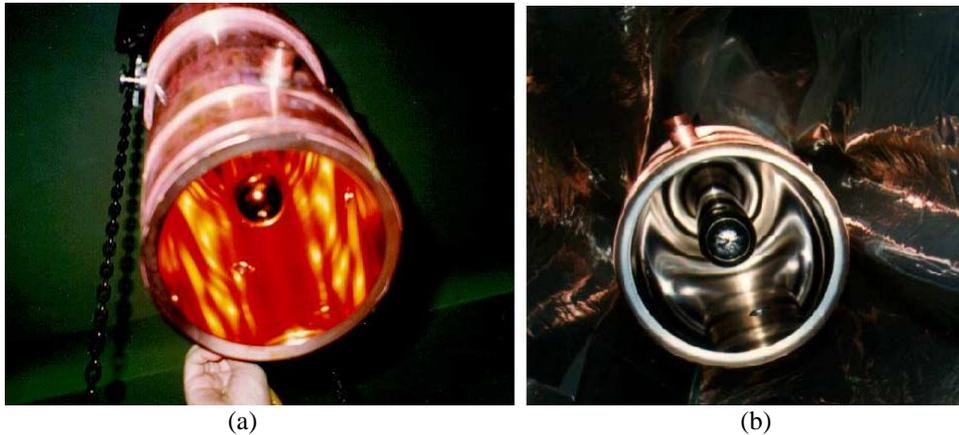
Fig. 3 QWR after electro-polishing (a) and after niobium coating (b)
