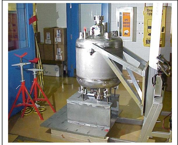
Figure 4. Cavity & Titanium Helium Vessel
