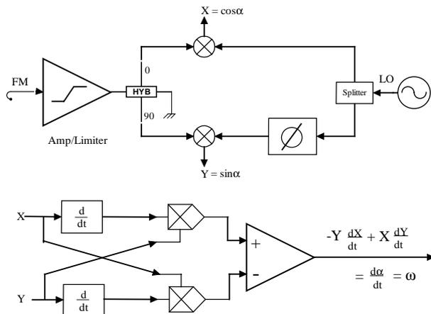
Figure 1: Cavity Resonance Monitor Block Diagram
