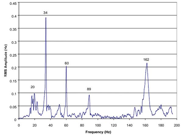
Figure 6: Cryomodule Impulse Response.
