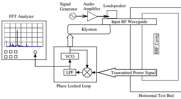
Figure 3: Swept Sine Test Setup.
