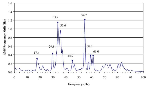
Figure 2: Cryomodule Response, Background Vibration.
