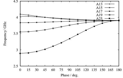
Figure 3: Dispersion curve of the first dipole passband of the cavities of shape A13 ... A25
