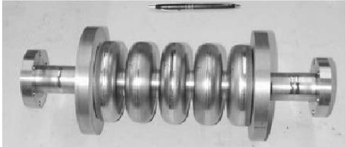
Figure 5: Five cell Niobium prototype transverse mode cavity.
