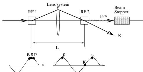
Figure 1: Kaon beam separation
