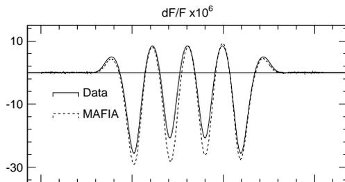
Figure 6: Results from bead pull measurements
