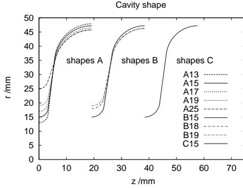
Figure 2: Half cell shapes of examined cavity designs
