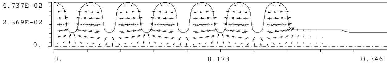
Figure 4: 13-cell cavity of shape C15, electric field of the  $\pi$ -mode ( $f = 3.8996$  GHz).
