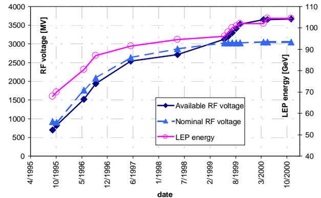
Figure 1.: Beam energy, available and nominal RF voltage from 1995 until 2000.
