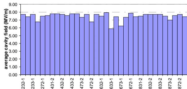
Figure 2: Average accelerating gradient of RF units with sputtered SC cavities after conditioning in 2000.
