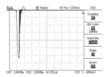
Figure 5: 130 kV Self-Break Crowbar Test
