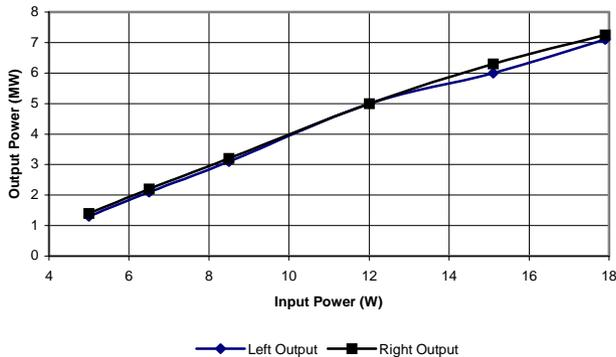
Figure 5. The measured drive curve.
