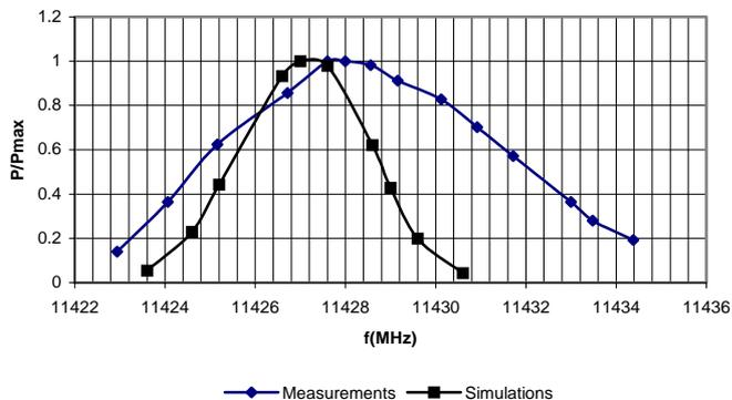
Figure 6. The measured and calculated magnicon bandwidth.
