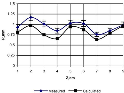
Figure 3. The beam envelope containing 95% of the beam current.
