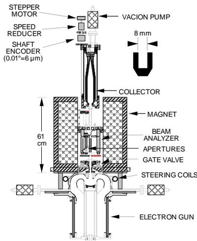
Fig. 2 Beam analyzer.
