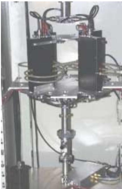
Figure 1: 900 W RF power amplifier assembly.
