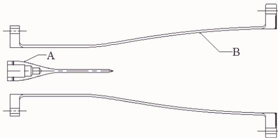
Figure 6: Schematic of Coaxial Uptaper (A - Inner transition, B -Outer taper)
