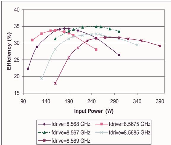
Figure 5: Theoretical drive curves for the 4 cavity circuit (for a number or different drive frequencies).
