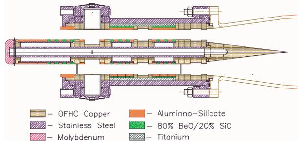
Figure 1: The Three cavity second harmonic circuit
