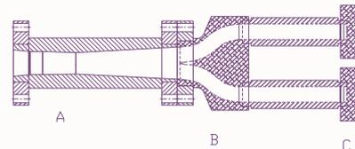
Figure 7: Schematic of part of new output waveguide system (A - circular to rectangular mode converter and rectangular taper; B - Bifurcation; C- Linear tapers into WR62 waveguides)
