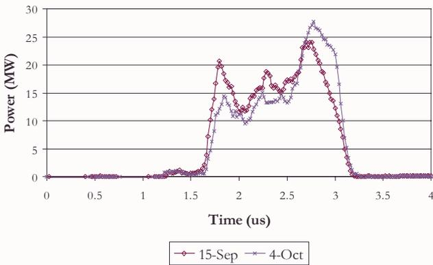
Figure 3: Output signals from 3 cavity gyroklystron, exhibiting nearly 30 MW of peak power.
