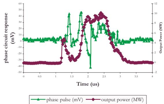
Figure 4: Comparison of output from phase correlation circuit and the output pulse
