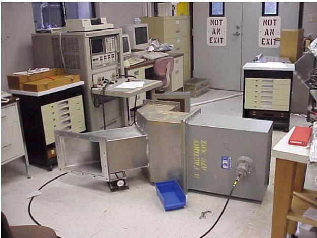
Figure 3: Test setup for adjusting matching for  $f_{RF}$  in modified mitre.
