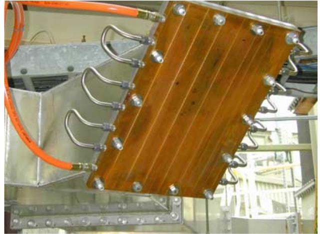
Figure 4: Finished waveguide load installed and in operation.
