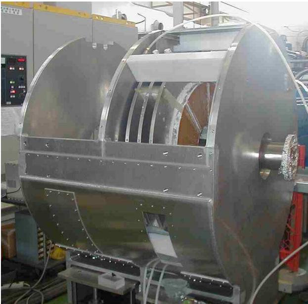
Fig. 3. A test cavity using an indirect-cooling method.
