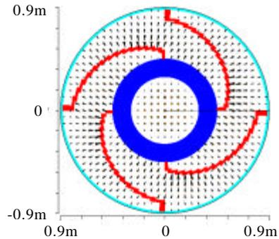
Fig. 5 The cross section of a ring-bar and the field
