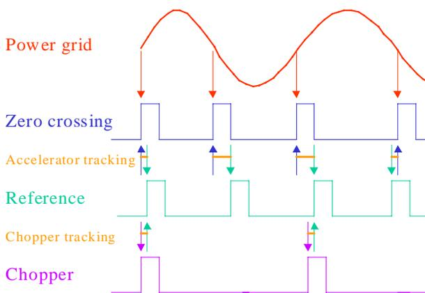
Figure 1. Timing waveforms and relationships.
