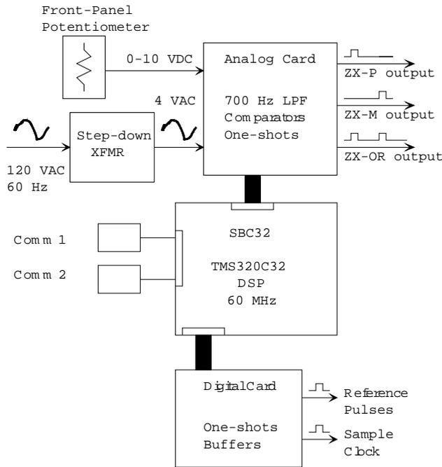
Figure 2. Block diagram of the timing-reference generator hardware.
