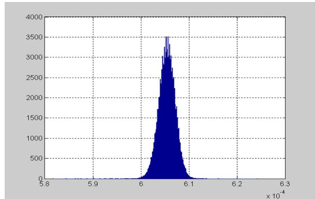
Figure 5. Level 7. Histogram of the time interval between the zero-crossing and reference output signals.
