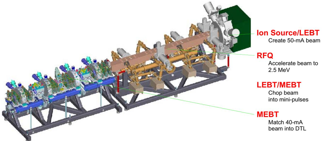
Figure 1. Layout of the SNS front-end beamline.
