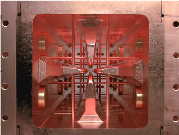
Figure 4: End-on view of the assembled RFQ Module #1 prior to the final brazing operation. The upstream ends of the four vanes are seen at the center, with  $\pi$ -mode stabilizers penetrating the vanes horizontally and vertically.
