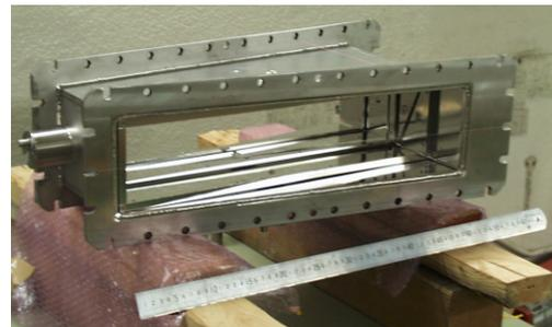
Figure 1: Beam Position Monitor (BPM).
