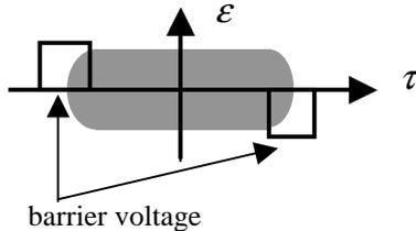
Figure 1: Barrier bucket RF system. Particles with positive energy errors slip to the right and are decelerated by the negative RF pulse; those with negative energy errors are accelerated by the positive pulse.
