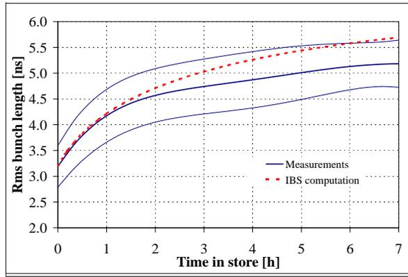
Figure 3: Rms bunch length increase during stores. The thick solid line shows the average, the thin solid lines the average plus and minus one standard deviation of a distribution.
