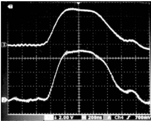
Figure 4: Observed kicker fields. The kicker current (lower, 200A/div) is measured with a current transformer. The current reaches its designed maximum value, 700A, within a 10-90% rise-time of 240nsec. The kicker field (upper, 500 mV/div) is measured with a search coil placed at the center of the kicker gap. The abscissa denotes 200nsec/div.
