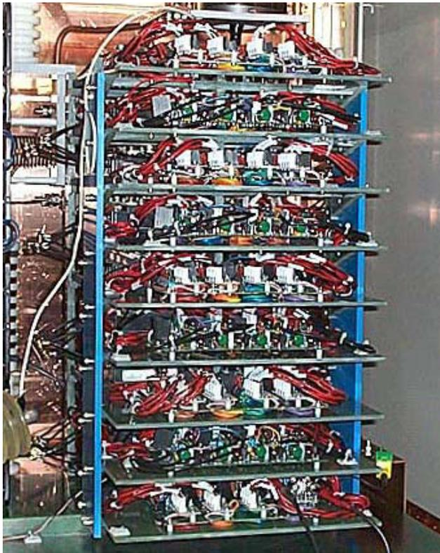
Figure 2: The subordinated-driving switching unit in the 1 kHz repetition power supply. The unit consists of nine layers of circuit boards, where each layer contains 16 IGBTs, 4 in series x 4 in parallel. The maximum switching voltage and current with this unit are 35kV and 700A. The height of the unit is about 60cm.
