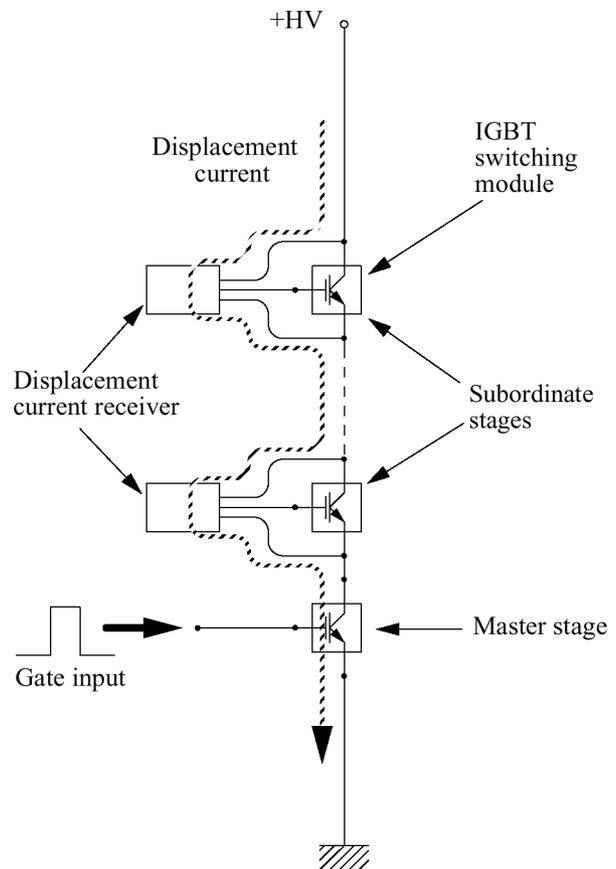
Figure 1: Principle of the subordinated gating system. Numbers of switching modules (in the figure, IGBTs) are connected in series. The gating signal is supplied only on the module closest to the earth potential, called the master-stage. The other stages are turned on subordinately to the master-stage.
