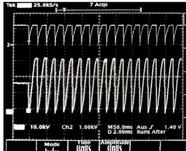
Figure 3: A confirmed result of the 1 kHz operation. The upper waveform is the master-stage voltage (1kV/div) and the lower waveform is the voltage across the switching unit in Fig. 2 (10kV/div). The applied DC voltage is 34 kV. The abscissa denotes 2msec/div.
