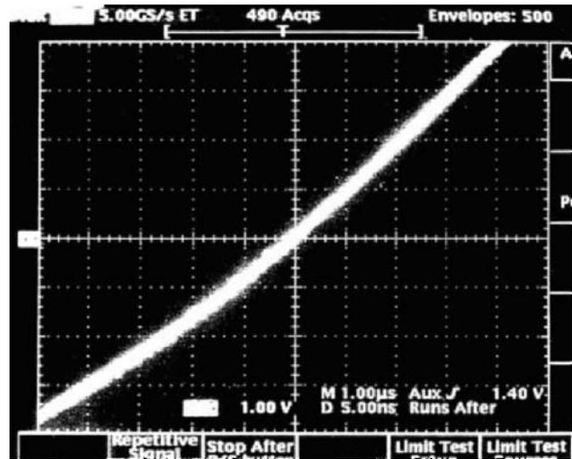
Figure 6: A measured result of the jitters in the output pulses. 500 pulses are overlapped in the above waveform. The charged voltage is 33 kV and the output current is 660 A. Both values are close to the designed maximum, 35kV/700A. The measurement is done at the output current of 100 A, which is at the center of the above figure. The jitters are found to stay within  $\pm 1$ nsec. The abscissa denotes 5 nsec/div.
