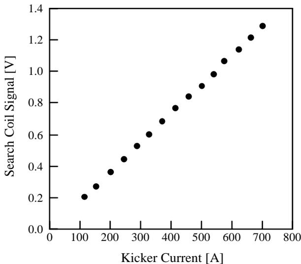
Figure 5: The output signal of the search coil with respect to the kicker current. The linear rise of the search coil signal indicates, as far as the measured range, there is no saturation within the MA (magnetic alloy) core by the magnetic field.
